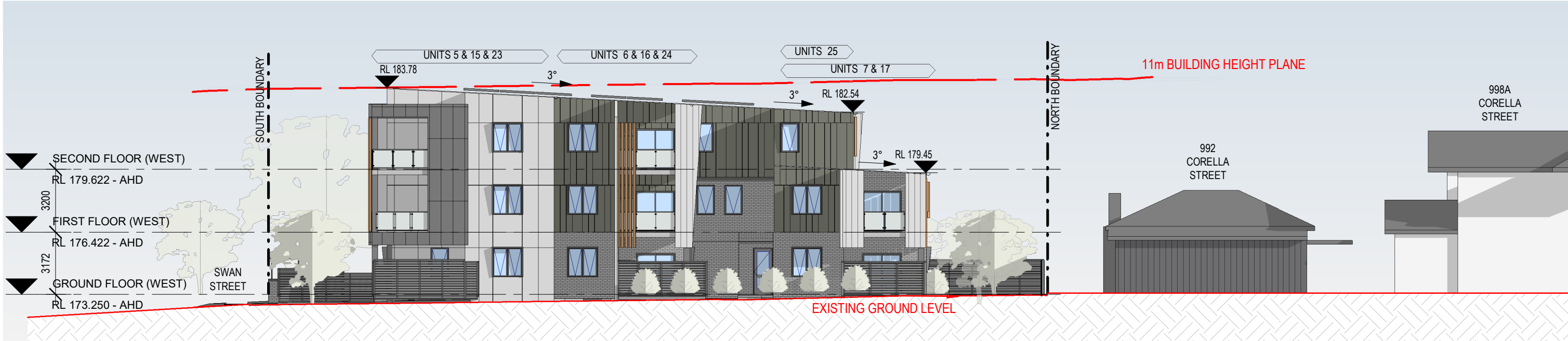
1 NOTIFICATION - EAST ELEVATION - (WEST BUILDING) SCALE 1 : 200
